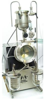
Myers Vacuum is based in Kittanning, PA where their team of engineers and technicians build Myers Vacuum is based in Kittanning, PA where their team of engineers and technicians build equipment, repair machinery, and make distillation units. These units are used for heat sensitive compounds and essential oils in a vacuum range of 1 to 80 X 10-3 Torr in the molecular weight range of 150 – 4000. Myers purchased the Molecular Vacuum Still line from CVC Products in 1990.
